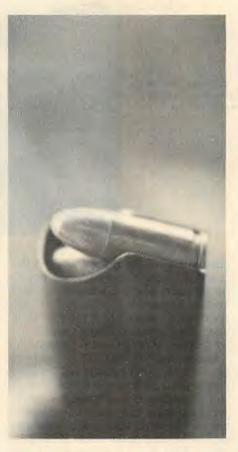
ABOVE: Magazine is double-column, squeezed into single column for feeding, a la P-35 Browning.
